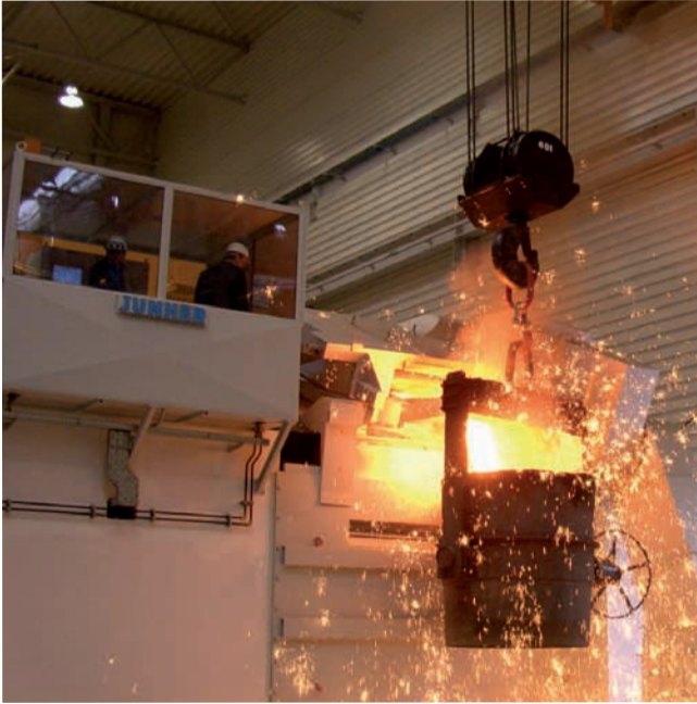
Powerful 9,000 kW cast iron melting furnace
