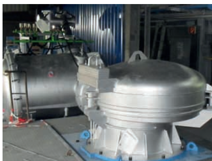
Coreless vacuum induction furnace
