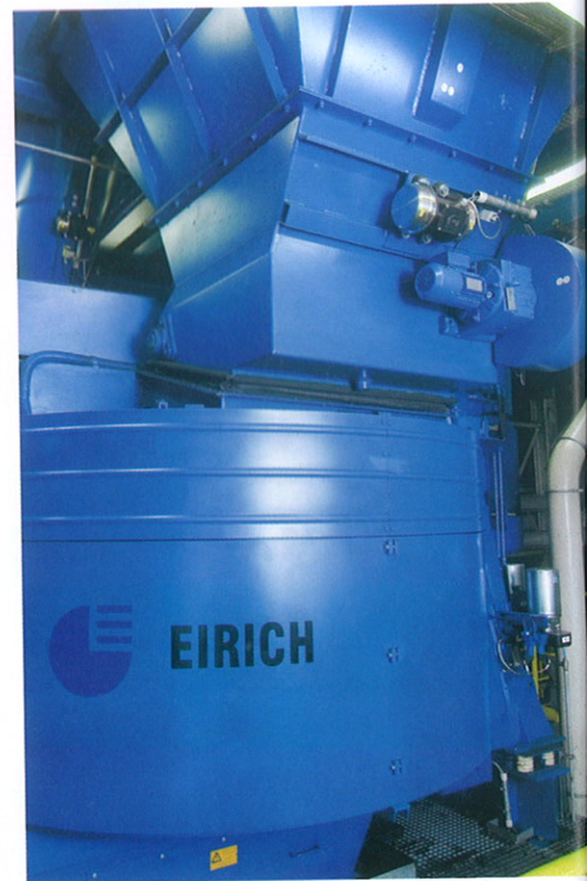
Figure 3: With the new turbo-mixer being the backbone of the sand preparation system, the capacity of the series production line in the main foundry shop at Olsberg could be markedly increased.
