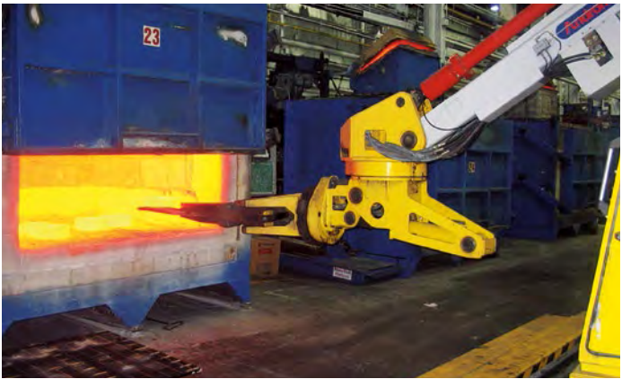
Andromat AMX 40 on a ring forging mill
