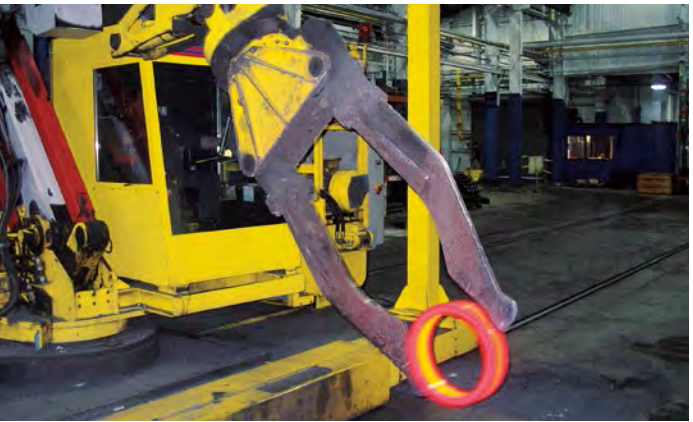
Wheel mounted Andromat AMX 40 in a forge
