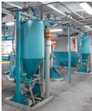
Scale cluster with water scale Control modules Moisture probe QualiMaster AT1 sand tester
