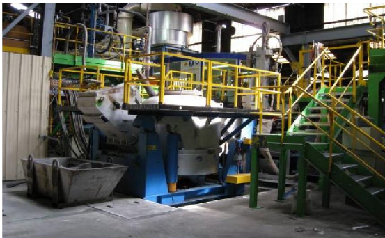
► 8-tonne pouring unit for spheroidal graphite cast iron
