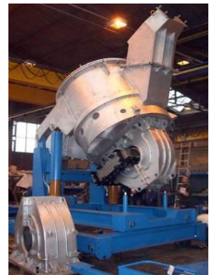
► 6-tonne-pouring unit for spheroidal graphite cast iron with bottom-mounted inductor (shop assembly photo)
