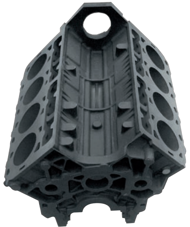
■ Engine block material: EN-GJL, mass: 150 kg
