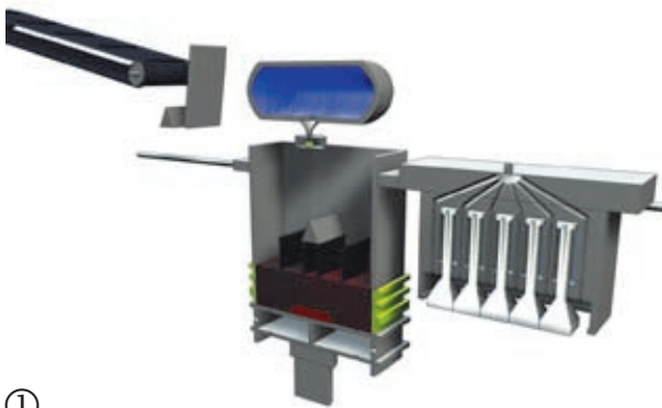
■ The sand is filled into the mould box to cover the pattern
