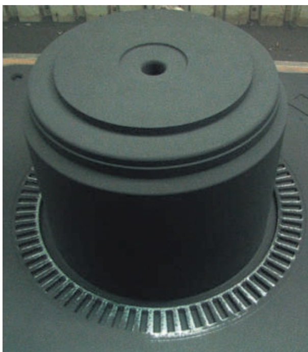
■ Mould example: Brake drum, Ø approx.: 500 mm
