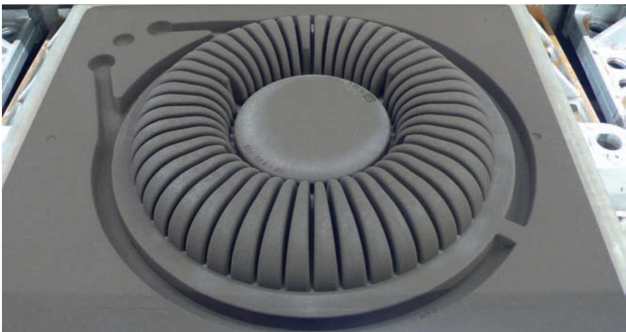
■ Mould example: Bottom Flask for a flow clutch, rib width 2.5 mm, dia. approx. 400 mm Previously made using sand cores, now with green sand mold insert. After the finishing pressure is applied an even mold is formed.
