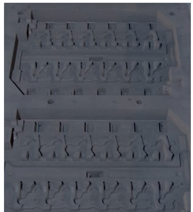
■ Mould example: Cylinder heads, flasksize: 1550 x 1100 mm
