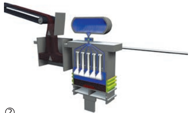
■ The SEIATSU AIRFLOW Squeeze Moulding Process is applied
