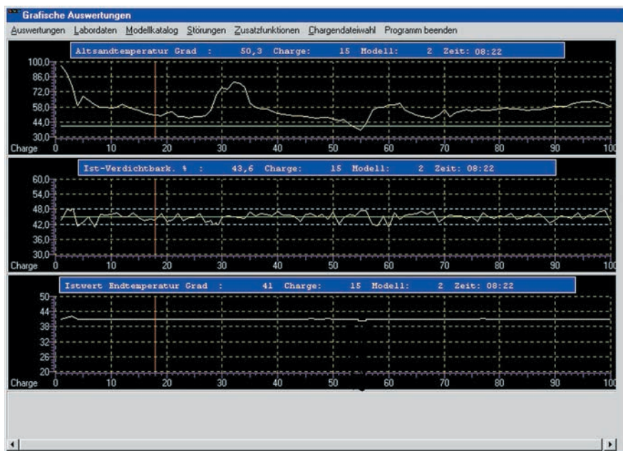
Fig. 8: SandExpert: View of the temperature curve of the return sand and the newly prepared molding material
