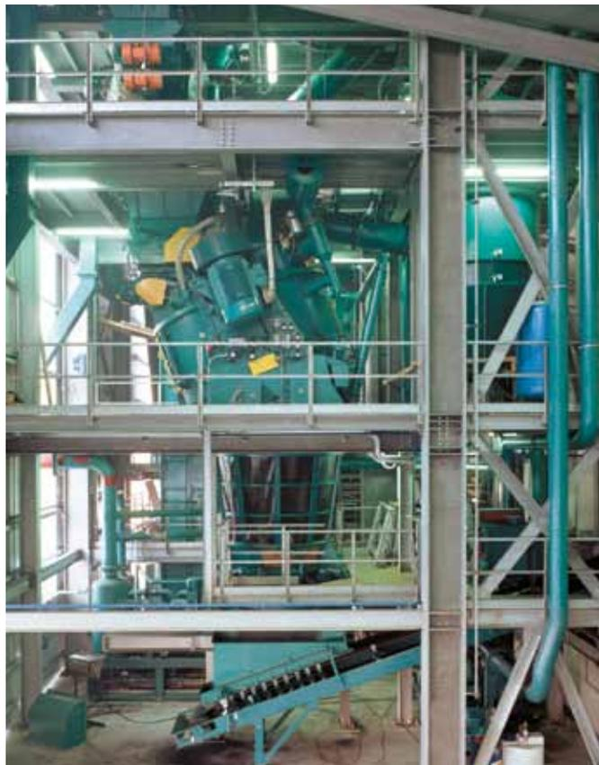
Fig. 4.1: EIRICH sand preparation system with EVACTHERM® RV32VAC mixer-cooler
