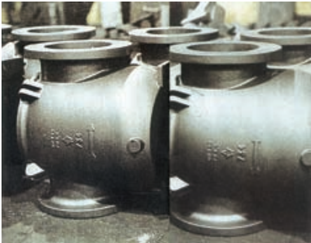
■ Filter case DN 200 for shipbuilding; material: GL-250, mass: 112 kg
