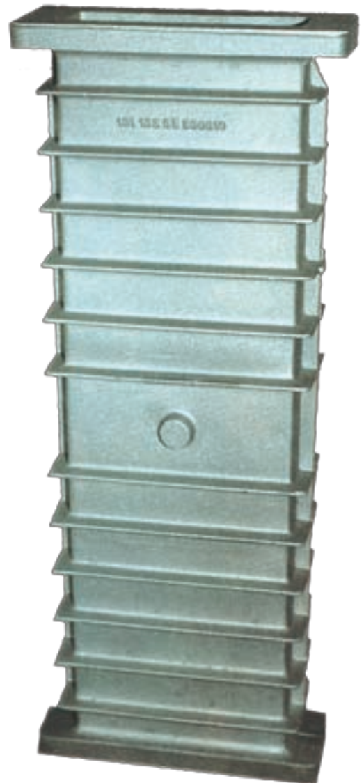
■ Cooler case with high demands to the gas tightness, material: G- \text{AlSi10Mg} wa, mass: 10 kg, dimensions: 710 x 300 x 120 mm
