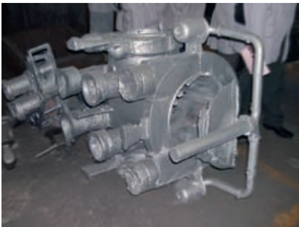
■ Valve body material: high alloy steel Japan
