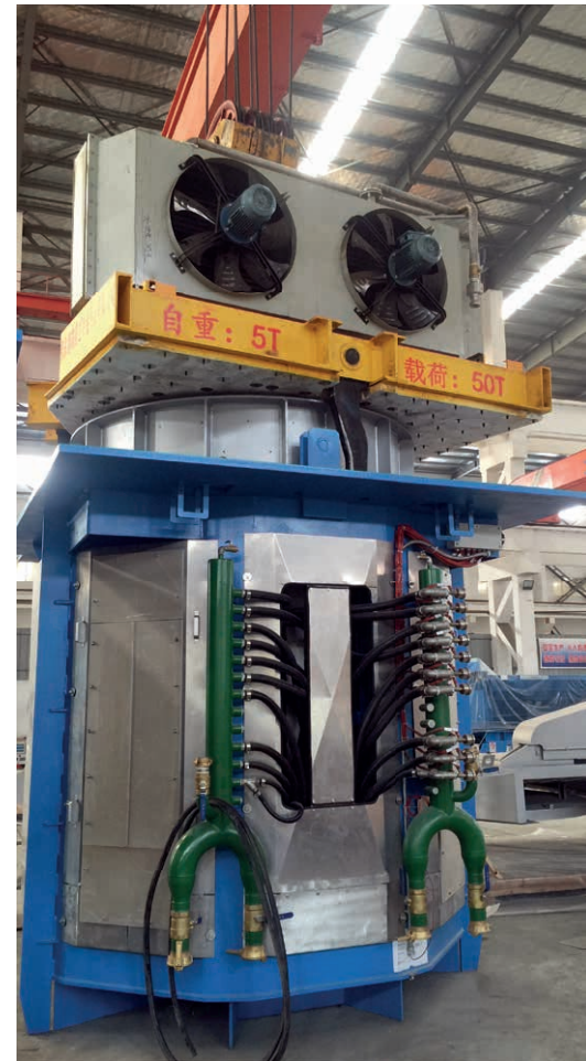
Hot-swap crucible assembly with mobile cooling system.
