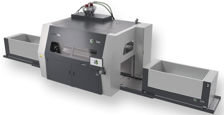
The S-MAX Pro™ impresses with its speed, reliability and precision. It is available as a stand-alone solution but is also scalable and can be connected by a network, that creates a fully automated production line, to realize the industrial serial production in 3D sand printing.
