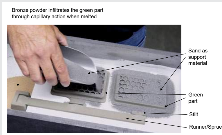
The bronze infiltration process (Courtesy The ExOne Company)
