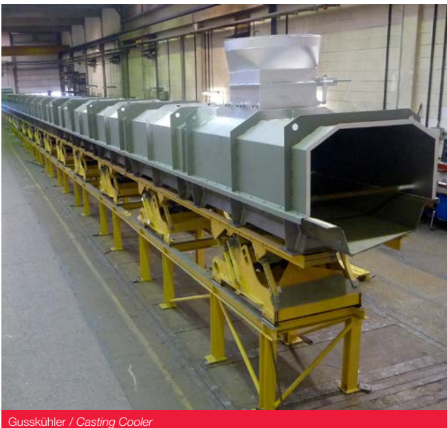
Gusskühler / Casting Cooler
