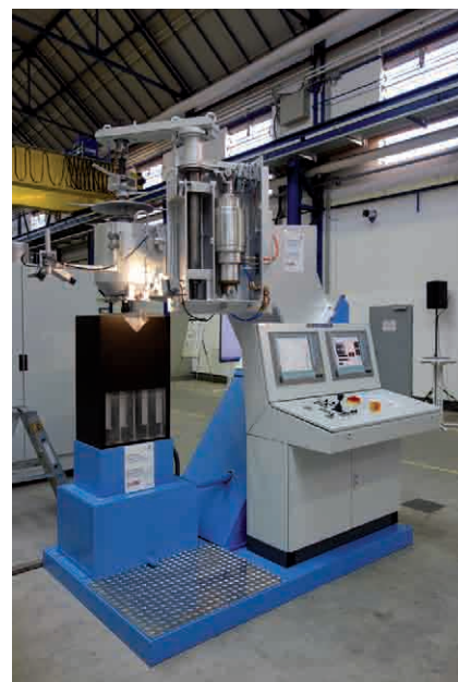
Figure 4: Trial setup comprising the new stopper actuator and Belysa camera system
