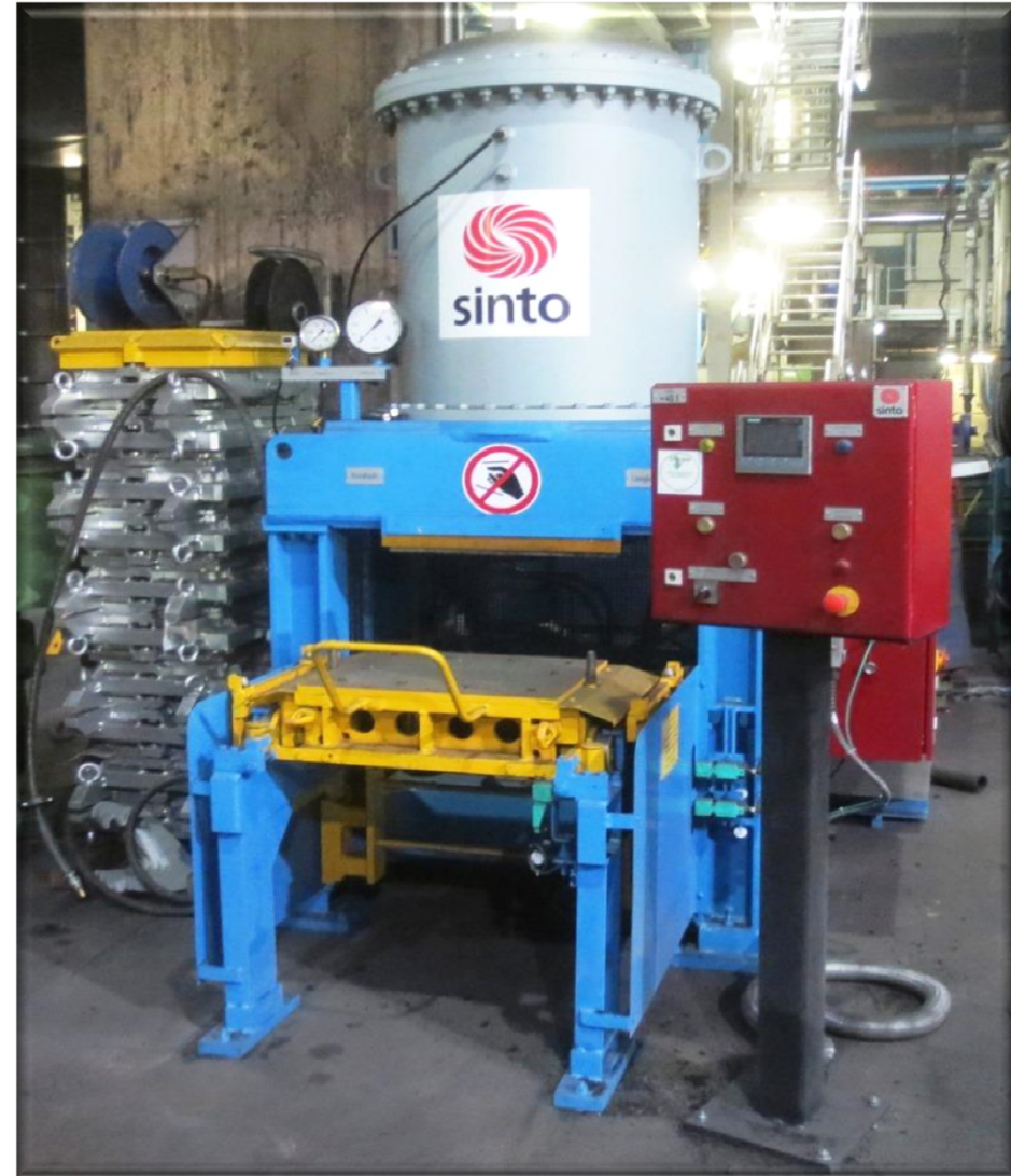
Picture: The moulding machine type “EFM-S“ is located in direct vicinity to the “big brothers“
