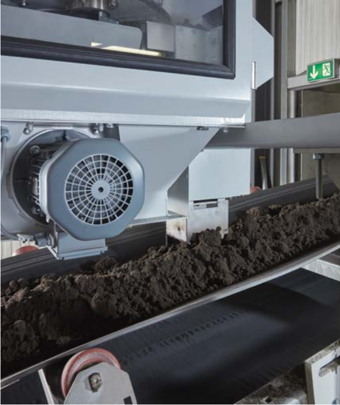
The QualiMaster AT1 inline tester takes the samples directly behind the mixer above the belt. An optional sample shredder can be integrated into the basic version AT1 Eco.
